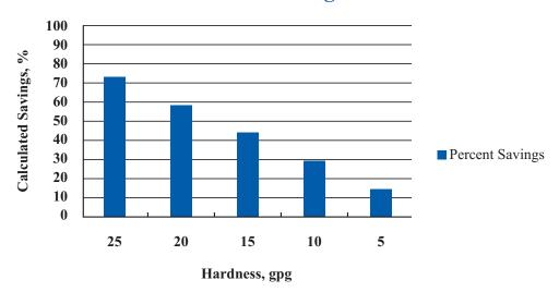
Detergent savings up to 70% was observed for dishwashing when softened water was used compared to hard water. Depending on the soil, hardness reduction was found to be up to 12 times more effective at soil removal than increasing detergent dose.
